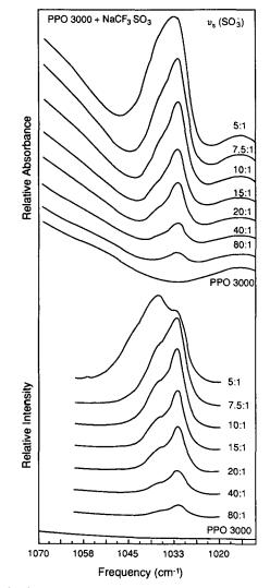
Figure 1 Comparison of room temperature parallel-polarized Raman scattering spectra and thin film i.r. transmission spectra of uncomplexed PPO and each of the PPO-LiCF<sub>3</sub>SO<sub>3</sub> complexes in the  $v_s(SO_3^-)$  spectral region
