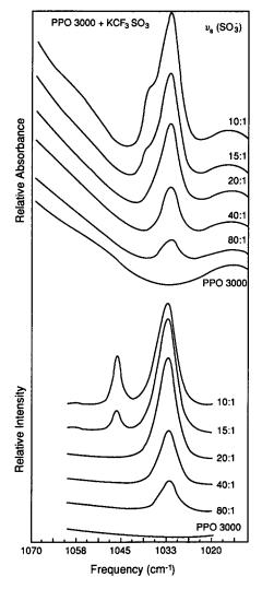
Figure 3 Comparison of room temperature parallel-polarized Raman scattering spectra and thin film i.r. transmission spectra of uncomplexed PPO and each of the PPO-KCF<sub>3</sub>SO<sub>3</sub> complexes in the  $v_s(SO_3^-)$  spectral region
