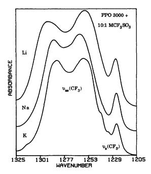
Figure 6 Thin-film i.r. transmission spectra of the 10:1 PPO-MCF<sub>3</sub>SO<sub>3</sub> (M = K, Na, Li) complexes in the  $v_{as}$  (CF<sub>3</sub>) spectral region
