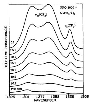
Figure 5 Thin film i.r. transmission spectra of uncomplexed PPO and each of the PPO-NaCF<sub>3</sub>SO<sub>3</sub> complexes in the  $v_{as}(CF_3)$  spectral region
