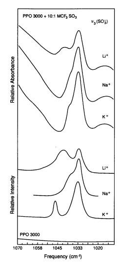
Figure 4 Comparison of room temperature parallel-polarized Raman scattering spectra and thin film i.r. transmission spectra of the 10:1 PPO-MCF<sub>3</sub>SO<sub>3</sub> (M = K, Na, Li) complexes in the  $v_s(SO_3^-)$  spectral region
